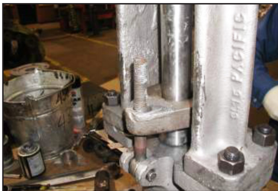
Without proper lubrication, the bolt tension will be off by as much as 40%.
