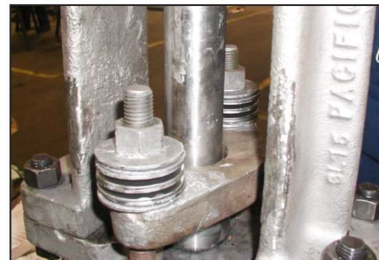
Threads, washers and disc springs are protected with Chesterton 725.
